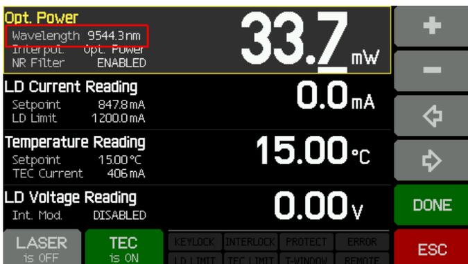
In Optical Power Interpolation mode, the value of the optical power is set by the user. The values of laser current and temperature are set, based on values stored in a calibration table, to maintain operation at the desired optical power. The wavelength or wavenumber are displayed to the left of the optical power.
