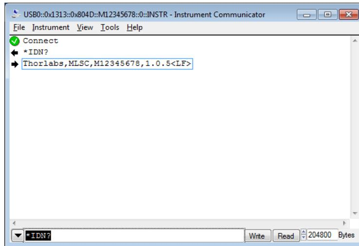
In above example, the \*IDN? command retrieves the identification information, which is being returned in the format "[manufacturer], [device name], [serial number], [firmware version]".
