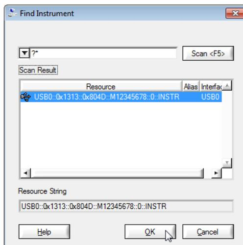
A list of available instruments appears. Select the MIR Laser System (can be recognized by serial number), then click 'OK'. The next screen allows to configure the USB connection and command line terminators. Click 'OK' to connect.
