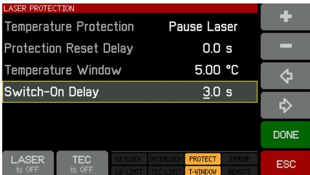
As required by Laser Safety Regulations, laser products of Class 3B and 4 are required to have a delay between switching on the laser and emitting radiation. The MIR Laser System has a minimum delay of 3 s and can be extended to 60 s.
