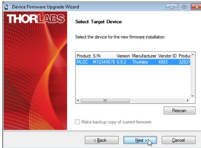
The DFU Wizard recognizes the connected DFU device. If you wish to save a backup copy of the present firmware, check the appropriate box.
