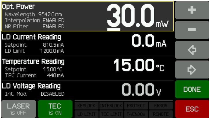
The settings can easily be changed - touch the desired parameter or value and the mode changes from read-only to set values.
