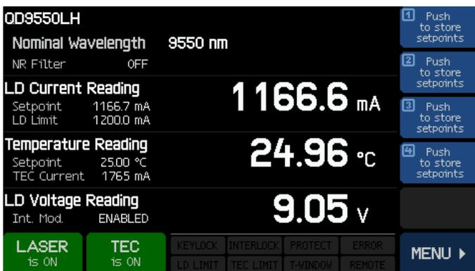
The factory default interpolation mode "OFF". The panel displays the nominal spectrum. Laser current and temperature can be set.
