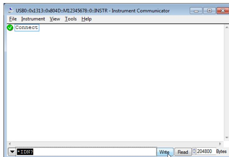
The Instrument communicator lists the sent command and the query result in the log panel:
