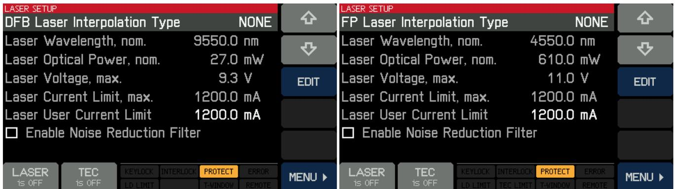
Laser Driver Setup - QCL-DFB Laser Head
