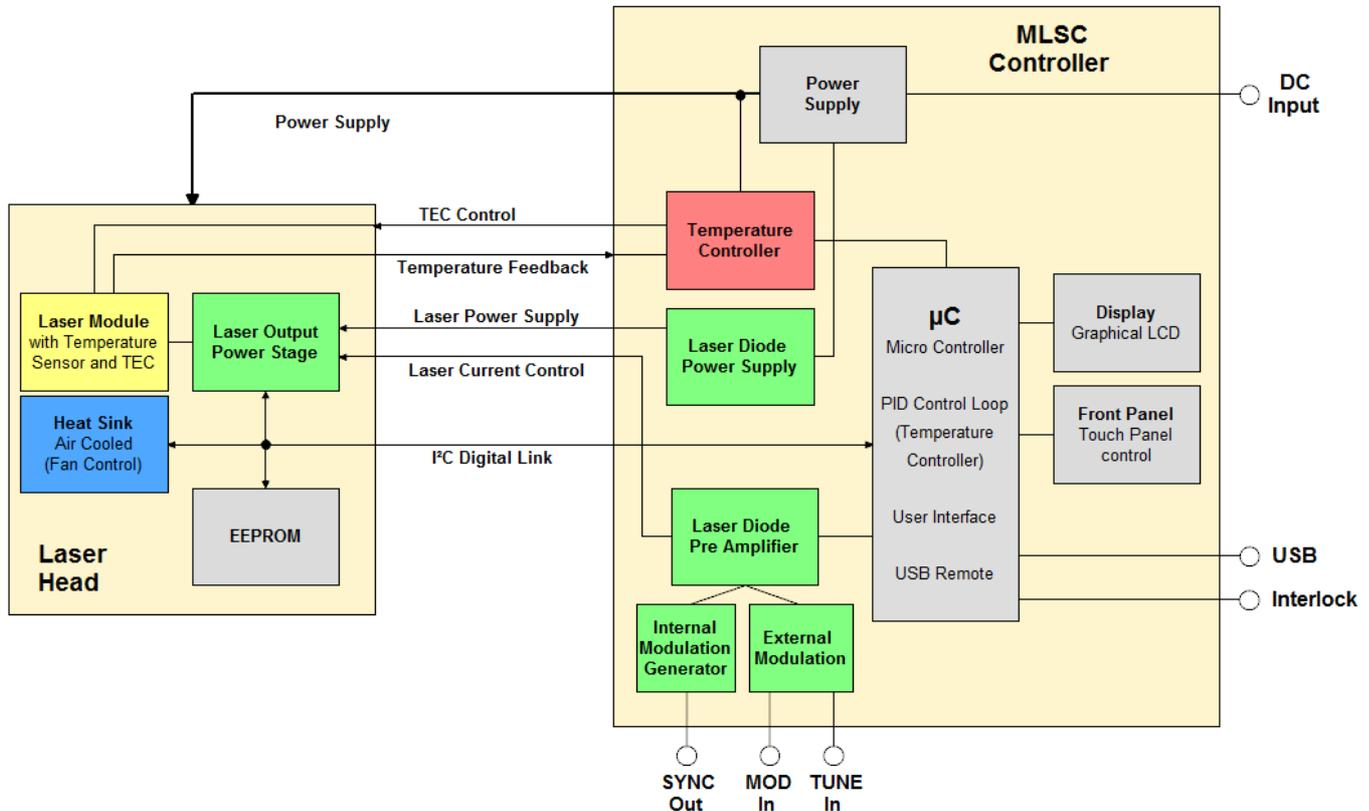
Block Diagram of the MIR Laser System
