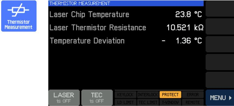
The MIR Laser System is designed to use the built-in thermistor for temperature sensing. Therefore, the resistance is measured and from this, the temperature can be calculated.
