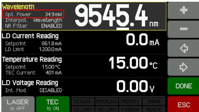
In Spectrum Interpolation mode, the wavelength or wavenumber is set by the user. The values of laser current and temperature are set, based on values stored in a calibration table, to maintain operation at the desired spectral output.
