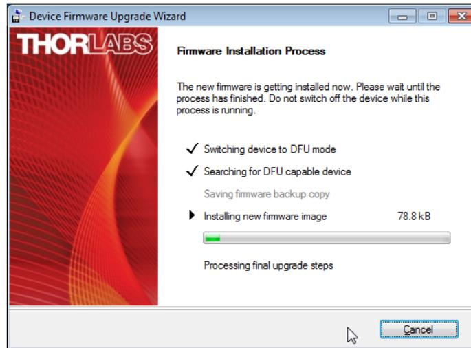
The DFU Wizard connects to the MLSC console and switches it to the DFU mode, which is reflected in a change of the LCD panel. Information on the DFU state and the process status is now displayed to the screen.
